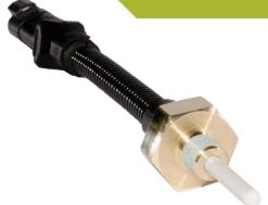
The **S287** is an active device designed to give an alarm signal if liquid falls below, or rises above, a preset level. It can be specified with a delay to eliminate false alarms due to turbulence and the flying lead enables customers to specify a suitable connector of their choice.
