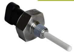
The **S298** is an active device designed to give an alarm signal if liquid falls below, or rises above, a preset level. It can be specified with a delay to eliminate false alarms due to turbulence.
