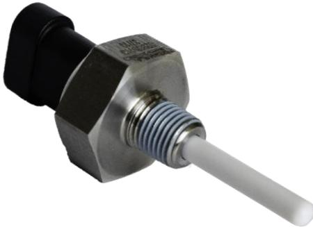
The **S298** is an active device designed to give an alarm signal if liquid falls below, or rises above, a preset level. It can be specified with a delay to eliminate false alarms due to turbulence.
