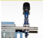
d. To free the centre rod from its end plug, carefully twist and pull the cut end from the sensor. Once outer tube is cut, you should be left with an exposed aluminium inner rod (see picture).
