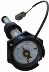
The **Model G/LL64** series vertical spiral gauge is an electromechanically operated liquid level gauge designed to continuously display the liquid level and provide a volt free contact as a high or low level alarm.
