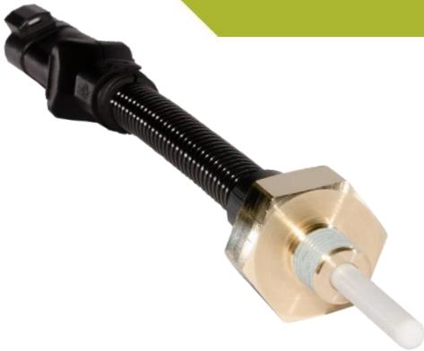
The **S287** is an active device designed to give an alarm signal if liquid falls below, or rises above, a preset level. It can be specified with a delay to eliminate false alarms due to turbulence and the flying lead enables customers to specify a suitable connector of their choice.
