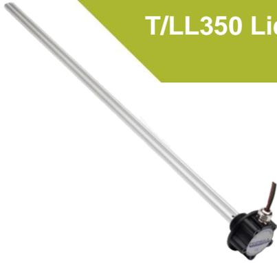
The **T/LL350** series is a range of highly advanced sensors for continuously measuring the contents of a tank. The unique feature of the T/LL350 is that it auto compensates when a liquid with a different dielectric constant is used. For example, if it is used in a tank of conventional diesel, then the user can refill with bio-diesel and the sensor will correct the output level automatically.
