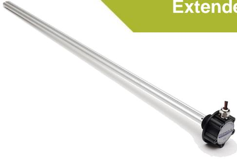
The **Model T/LL360** is an extended temperature range variant of the T/LL350 series of highly advanced sensors for continuously measuring the contents of a tank. Capable of operating at temperatures as low as  $-40^{\circ}\text{C}$  the T/LL360 series auto compensates when a liquid with a different dielectric constant is used. For example, if it is used in a tank of conventional diesel, the user can refill with biodiesel and the sensor will correct the output level automatically.
